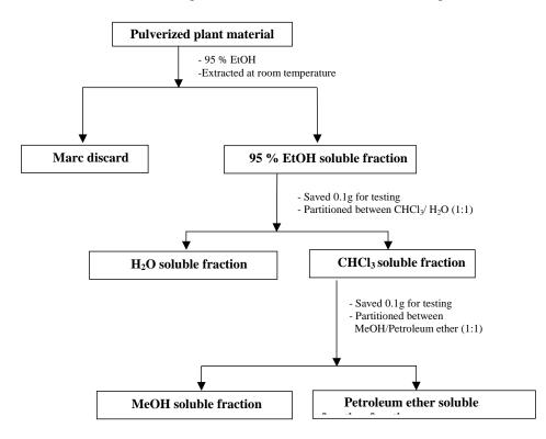
fractions derived in the whole process were transferred into vials and used in a two- choices cowpea weevil bioassay (Abdullahi *et al.*, 1995). The flow chart for the extraction and partition processes is as shown:
